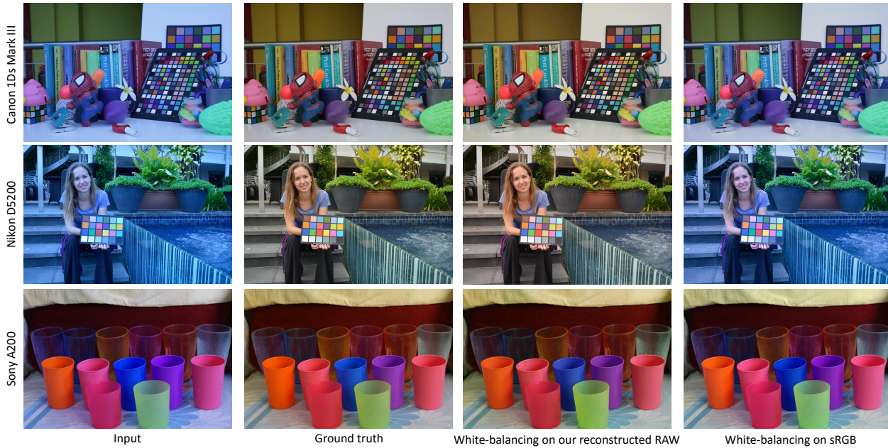
Figure 8. This figure shows examples on correcting white-balance for different cameras: a Canon 1Ds Mark III, a Nikon D5200, and a Sony \alpha 57. The first column is the input images captured under the wrong white-balance settings; the second column shows the ground truth images captured under the proper settings. The third column displays the results applied the white-balance correction on our reconstructed RAW images. The final column shows the results applied the white-balance correction directly on the sRGB-JPEG images.
